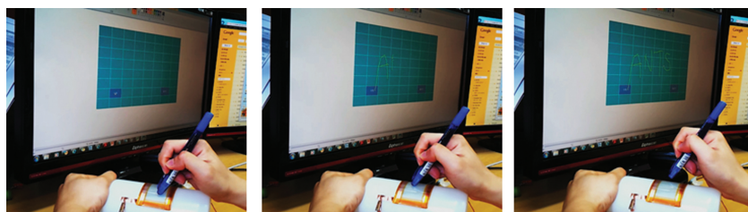
Figure 8. Demonstration of a bendable touch screen on a non-flat surface. Letters “ANTS” were written.
